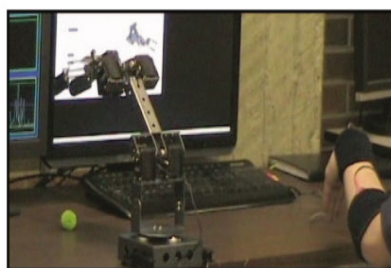
(b) Prosthesis Limb Controller for AX-12 Smart Arm. Source: (Pilarski et al. , 2011).
