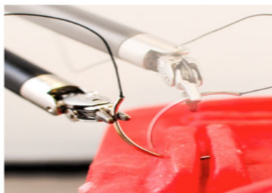
(a) Suture Tying on a Surgical Da Vinci Research Kit. Source: (Laskey et al. , 2016).
