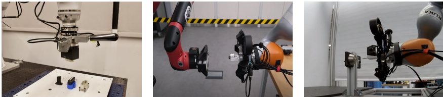
(a) NIST board insertion (b) Moving HDMI Insertion (c) Key-lock insertion
