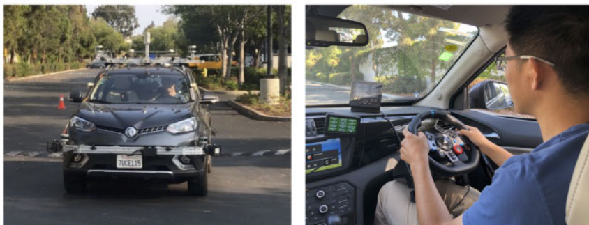
Figure 11.6: Test vehicle (left) and expert driver interface (right). Source: (Kelly et al. , 2019).
