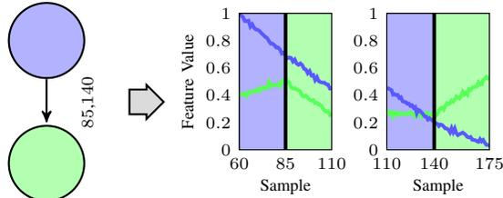
(c) One classifier is created for each node in the graph. Only the features of the previous primitive and its possible successors are used for training. In this exemplary transition from the upper sequence graph, the red primitive is not involved and hence its feature is not used.
